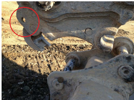
lack of manual safety pin
